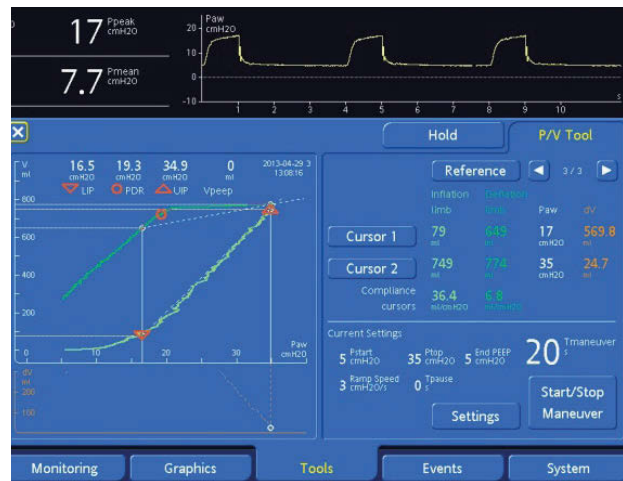
A cursor function permits graphical analysis of the curve, including identification of inflection points
