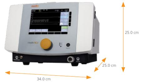
The medin-NC3® CPAP driver is used in combination with the Medijet® nCPAP generator to administer CPAP therapy or with a suitable Nuflow® nasal cannula to administer High Flow therapy to premature infants and newborns. The medin-NC3® must be used under the supervision of expert, specially trained staff in a clinical setting or during intrahospital transport, and the patient's oxygen saturation must be monitored at the same time.
